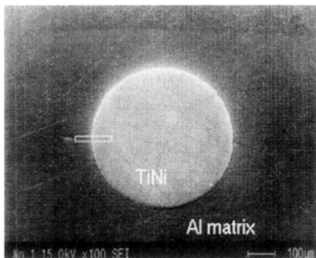
Fig. 4 SEM micrograph of the TiNi/Al6061 SMA composite
